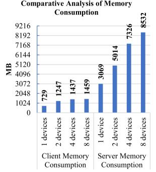
**Fig. 10** Performance evaluation of memory consumption by client and server devices of FEDDBN-IDS Model with D = 1
