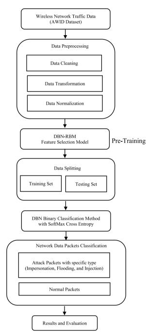
Fig. 4 Proposed scheme of the DBN method for training the local models
