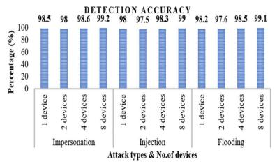
Fig. 11 Attack-specific detection accuracy of FEDDBN-IDS with D = 0
